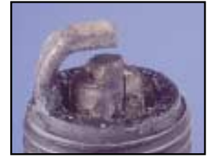
4. DETONATION 4. DETONATION 4. DETONACION
