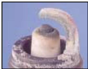
5. WORN OUT 5. DETERIORATION 5. DETERIORO
